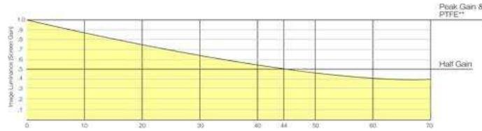
Graphite 100 is an acrylic rear projection screen material formulated to combine a 30% neutral density gray acrylic substrate with an above unity gain and wide angle optical coating. Graphite 100 is a high resolution, unity gain screen with good off axis performance and reasonable resistance to ambient light in the viewing area. Graphite 100 is best utilized with medium throw or longer projection light paths.
