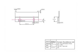
The only thing that is optional (free of charges) is to opt for 4 snap-in brackets instead of 2 Z-brackets and 2 snap-in brackets. This option is for integrating the screen in a recessed cabinet, when there is no room around it.
